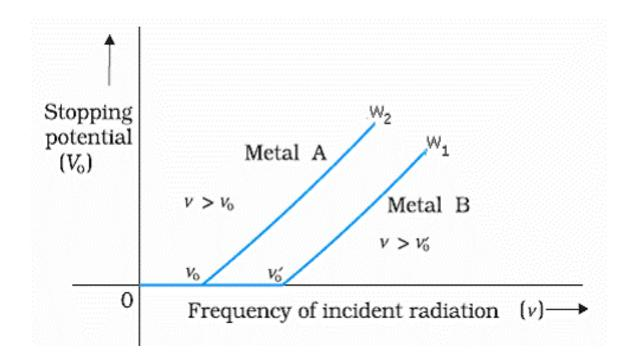
**Conclusion:** Above the threshold frequency, the stopping potential is directly proportional to the frequency of incident radiation.
