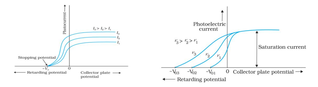
**Conclusion**: Above the threshold frequency, the stopping potential or equivalently the maximum kinetic energy of the photoelectrons is directly proportional to the frequency of incident radiation, but is independent of its intensity.
