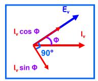
The component  $I_v \cos \Phi$  generates power with  $E_v$ .
