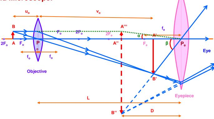
Objective: The converging lens nearer to the object.
