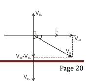
$$\begin{split} V_{o} &= \sqrt{\left(V_{oC} - V_{oL}\right)^{2} + V_{oR}^{2}} \\ &= \sqrt{\left(I_{o} X_{C} - I_{o} X_{L}\right)^{2} + \left(I_{o} R\right)^{2}} \\ &= I_{o} \sqrt{\left(X_{C} - X_{L}\right)^{2} + R^{2}} \end{split}$$
