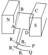
(b) Field magnet:- It is a strong permanent magnet with concave pole pieces. Armature coil is made to rotate about an axis perpendicular to the field lines between the pole pieces.
