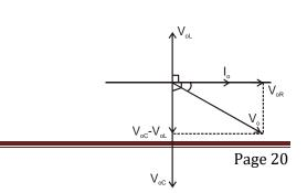
$$V_{o} = \sqrt{(V_{oC} - V_{oL})^{2} + V_{oR}^{2}}$$
