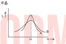
If the figure shows resonance curves for two circuits A and B then  $Q_A > Q_B$ (As resonance curve of A is sharper)
