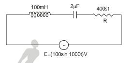
**Solution :**  $x_{L} = \omega L = (1000 \times 100 \times 10^{-3}) \Omega = 100 \Omega$
