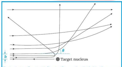
Trajectory of α-particles in the coulomb field of a target nucleus. The impact parameter, b and scattering angle  $\theta$  are also depicted.
