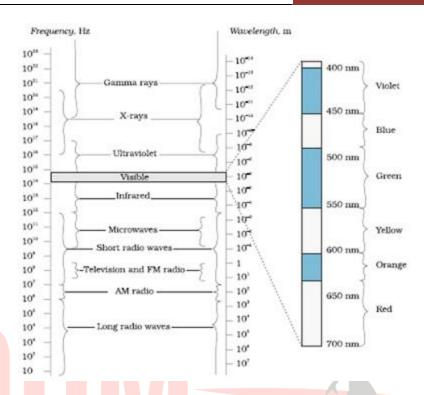
The electromagnetic spectrum, with common names for various parts of it. The various regions do not have sharply defined boundaries.
