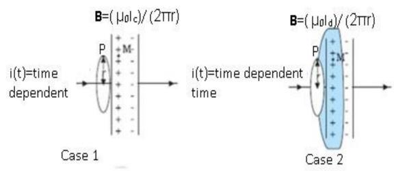
Consistent values of **B** at the same point of the same setup even though different amperial loops are considered.
