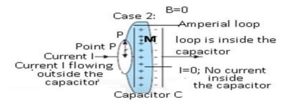
As there is no current flowing inside the capacitor, therefore I = 0
