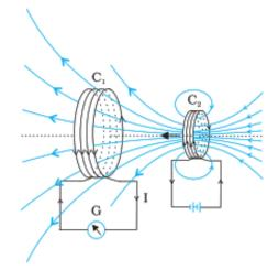
Here the bar magnet is replaced by a second coil  $C_2$
