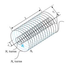
The magnetic field inside the primary solenoid
