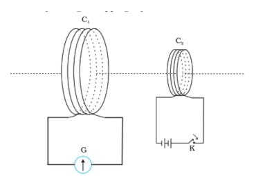
Here relative motion is not an absolute requirement coils C<sub>1</sub> and C<sub>2</sub> held stationary
