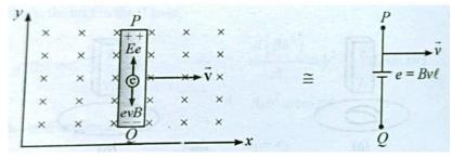
From the diagram, the magnetic force on the free electrons  $\vec{F}_m = -2(\vec{v} \times \vec{B})$  move towards end Q within the rod, hence end Q becomes –ve w.r.t P.
