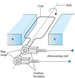
(d) Brushes – Two flexible metal rods which kept pressing against the slip ring. They are used to pass the current from armature to external resistance R.
