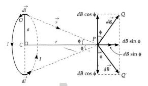
The magnetic field dB can be resolved into two rectangular components  $dB \sin \phi$  and  $dB \cos \phi$ . The components perpendicular to the axis of the loop will be equal and opposite and will cancel out. Their axial components will be in the same direction, so added up.
