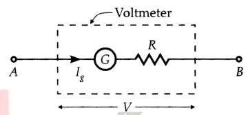
through the voltmeter and so the current through the circuit element decreases. This decreases the potential difference required to be measured. To avoid this, the voltmeter should be designed to have very high resistance. In fact, an ideal voltmeter should have infinite resistance.
