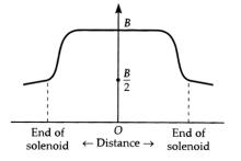
The figure shows the variation of the magnetic field on the axis of a long straight solenoid with distance x from its center.
