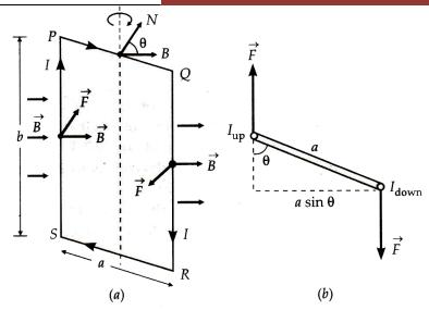
resultant is zero. According to Fleming's left rule, the side PS experiences a normal inward force equal to NIbB while the side QR experiences an equal normal outward force. The two forces on sides PS and QR are equal and opposite. They form a couple and exert a torque given by.
