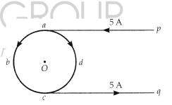
$$\textbf{Solution:-Here,} \ \ I_{abc} = I_{adc} - 2.5A, r = Oa, Ob = Oc = Od = 5cm = 5 \times 10^{-2} m$$
