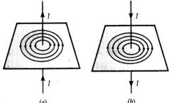
Rules for finding the direction of the magnetic field due to straight current-carrying conductor:-
