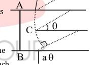
Here intensity at any point is due to the contribution of all points of the wavefront AB. If we imagine two parts of the wavefront then for each point of upper half i.e AC there exist a point on lower half BC at a distance a/2.
