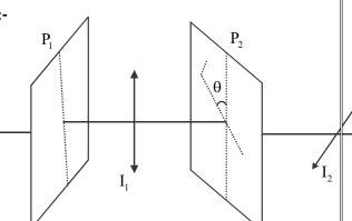
Unpolarised light of intensity  $I_0$  is incident of  $P_1$  called as the polarizer
