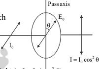
If the incident light is unpolarised, then the intensity of transmitted light is  $I = I_0 \langle cos^2 \theta \rangle$
