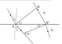
r = The angle of refraction  $\angle AB'A'$  light, travelling from rarer medium of refractive index  $n_1$  to denser medium of refractive index  $n_2$ .
