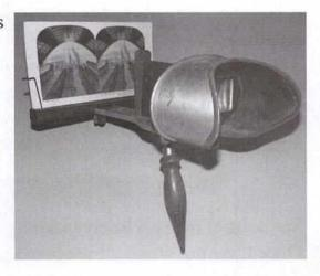
It had a handle at the bottom. There was a frame that had a pair of flint glasses fixed to it. One had to hold the handle and peer through these. The picture stood in a holder behind the frame. It was not a single picture, but two pictures placed side by side on a card. They looked identical, but that was not really the case. It was the same scene, but shot with a camera with two lenses.
