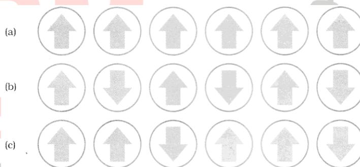
Schematic alignment of magnetic moments in (a), ferromagnetic (b) antiferromagnetic and (c) ferrimagnetic.
