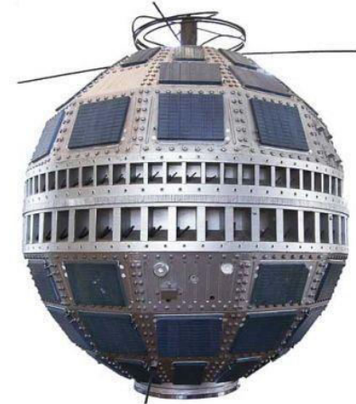
TELSTAR First communication satellite
