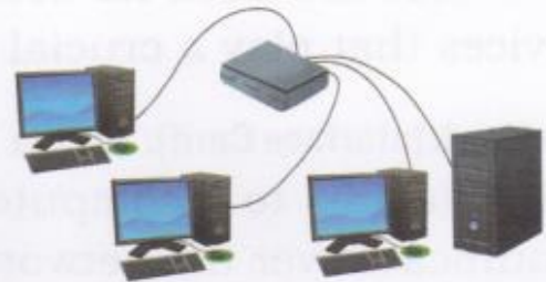
▲ Fig. 1.26 Networking using a hub
