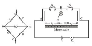
Its unit is  $\Omega$ -m (ohm-meter). To measure its resistivity, we use a meter bridge. The working of a meter bridge is based on Wheatstone bridge principle. The circuit shown is called
