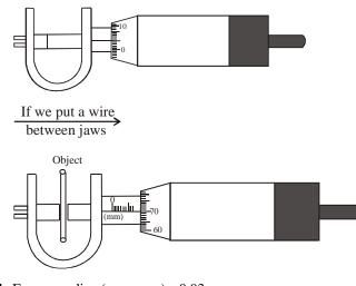
Sol. Excess reading (zero error) = 0.03 mm It is giving 7.67 mm in which there is 0.03 mm excess reading, which has to be removed (substracted) so actual reading = 7.67 - 0.03 = 7.64 mm
