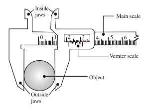
Suppose the size of one main scale division (M.S.D.) is M units and that of one vernier scale division (V. S. D.) is V units. Also let the length of 'a' main scale divisions is equal to the length of 'b' vernier scale divisions.
