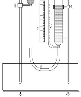
**Procedure :** Following steps are used in the experiment. (a) Hold the vibrating tuning fork at the open ,end of the column and start increasing the length of the air column by adjusting the height of reservoir.
