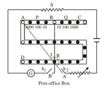
The wire whose resistance (S) is to be determined is connected in the arm CD. The galvanometer G is connected between Band D through the key  $k_2$  and the cell is connected between A and C through the key  $k_1$ .
