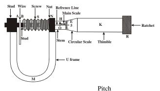
Least Count =  $\overline{\text{Total no. of divisions on the circular disc}}$ where pitch is defined as the distance moved by the screw head when the circular scale is given one complete rotation, i.e.
