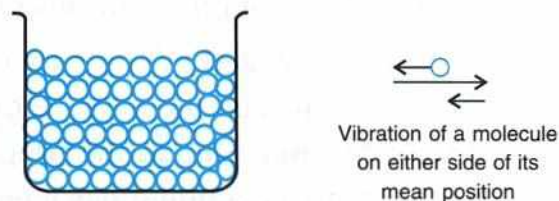
Fig. 1.3 Molecules of a solid are arranged closely and in a definite manner, not free to move about
