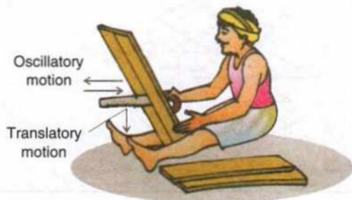
Fig. 2.16 The translatory and oscillatory motions of a carpenter's saw
