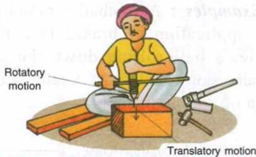
Fig. 2.15 Translatory and rotatory motions of a drill used by a carpenter
