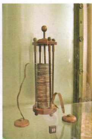
The battery built by Alessandro Volta
