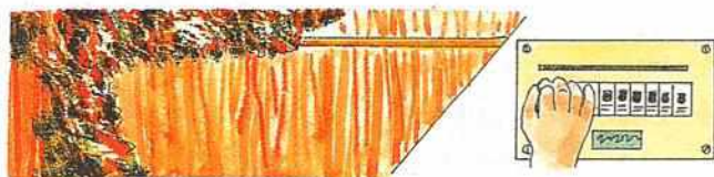
Fig. 3.10 Put off the main switch in case of an electric fire.
