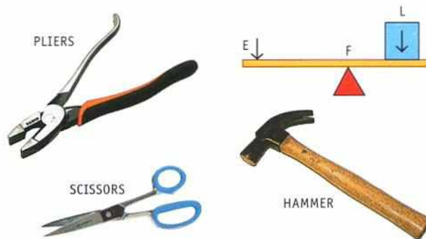
Fig. 11.4 Examples of first-class levers
