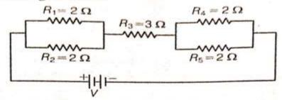
Sol. In the given circuit,  $R_1$  and  $R_2$  are in parallel. So, their equivalent resistance R' is given by
