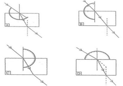
For measuring the angle of incidence, he must position the protractor in the manner shown in the figure:
