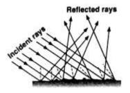
Reflecting surface is rough and the reflected rays from parallel incident rays are not parallel.
