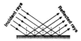
Reflecting surface is smooth and the reflected rays from parallel incident rays are also parallel.
