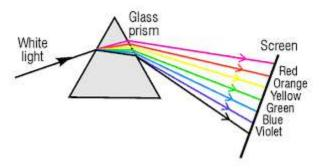
Cauchy's formula ;  $\mu = A + \frac{B}{\lambda^2} + \frac{C}{\lambda^4} + \dots$  we can conclude that material has minimum
