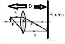
Solutions of this quadratic equation represents two positions ( $x_1$  and  $x_2$ ) of lens for producing image on the screen . As given ,  $x_2 - x_1 = d$
