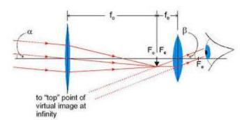
(ii) The ray diagram of refracting type stronomical telescope for final image at least distance of distinct vision is shown below .
