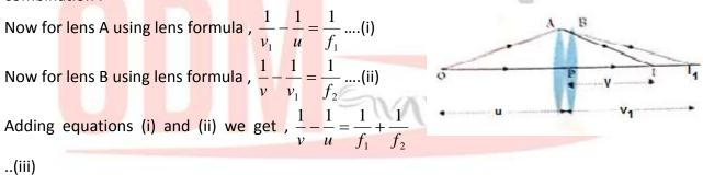
Since u = object distance for the combination and v = image distance of combination , Hence for the combination ;  $\frac{1}{v} - \frac{1}{u} = \frac{1}{f}$  ...(iv)
