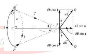
Consider a current element  $d\vec{\ell}$  at the top of the loop. It has an outward coming current. It  $\vec{s}$  is the position vector of point P relative to the element  $d\vec{\ell}$ , then from Biot-Savart law, the field at point P due to the current element is
