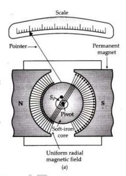
restoring torque and serve as current leads. A light aluminum pointer attached to the coil measures its deflection on a suitable scale.
