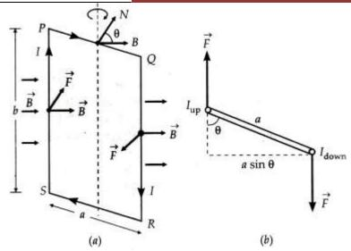
resultant is zero. According to Fleming's left rule, the side PS experiences a normal inward force equal to NIbB while the side QR experiences an equal normal outward force. The two forces on sides PS and QR are equal and opposite. They form a couple and exert a torque given by.
