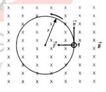
shown by small crosses. A charge +q is projected with a speed v in the plane of the paper. The velocity is perpendicular to the magnetic field. A force F=qvB acts on the particle perpendicular to both  $\vec{v}$  and  $\vec{B}$ . This force continuously deflects the particle sideways without changing its speed and the particle will move along a circle perpendicular to the field.
