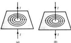
with the wire at the center and in a plane perpendicular to the wire. (A line of force is a curve, the tangent to which at any point gives the direction of the magnetic field at that point). If the current flows upwards, the lines of force have an anticlockwise sense and if the current flows downwards then the lines of force have a clockwise sense.
