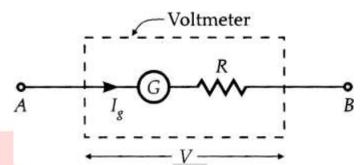
through the voltmeter and so the current through the circuit element decreases. This decreases the potential difference required to be measured. To avoid this, the voltmeter should be designed to have very high resistance. In fact, an ideal voltmeter should have infinite resistance.
