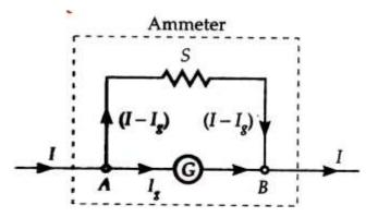
current, an ammeter should have zero resistance. So ammeter is designed to have very small effective resistance. In fact, an ideal ammeter should have zero resistance. An ordinary galvanometer is a sensitive instrument. It gives full-scale deflection with a small current of few microamperes. To
