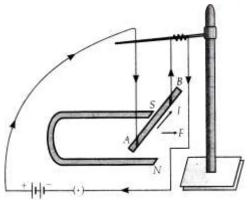
it current is passed through the rod from A to B, the rod gets deflected to the right. If we reverse the direction of the current or interchange the poles of the magnet, the deflection of the rod is also reversed. The direction of force is perpendicular to both the current and the magnetic field and is given by Fleming's left-hand rule.
