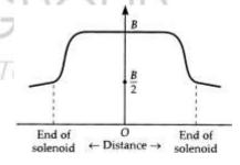
The figure shows the variation of the magnetic field on the axis of a long straight solenoid with distance x from its center.
