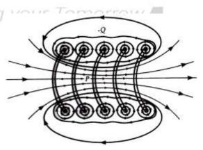
various turns of the solenoid, current enters the plane of paper at points marked  $\oplus$  and leaves the plane of paper at points marked  $\Box$ . The magnetic field at points close to a single turn of the solenoid is in the form of concentric circles like that of a straight current-carrying wire. The resultant field of the solenoid is the vector sum of the field due to all the turns of the solenoid. Obviously, the fields due to
