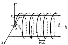
The velocity  $\vec{v}$  can be resolved into two rectangular components
