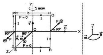
Fleming's left-hand rule, are perpendicular to the plane of the paper, one pointing outwards  $\Box$  and other inwards  $\otimes$  as shown in the figure.
