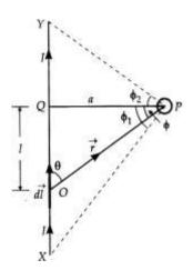
According to Biot-Savart law, the magnitude of the field  $d\vec{B}$  due to the current element  $d\vec{\ell}$  will be.
