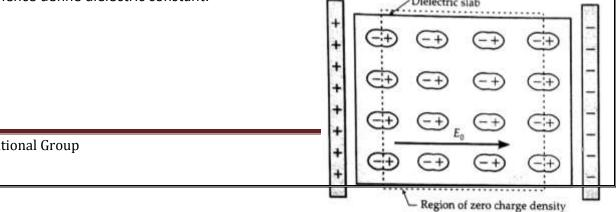
Solution:- Consider a rectangular dielectric slab placed in a uniform electric field  $\vec{E}_0$  acting parallel to two of its faces.
