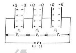
$$V = V_1 + V_2 + V_3$$
