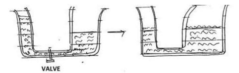
When the value is open, the level in both the vessels become equal but the volume of liquid in the right vessel is more than the left vessel.
