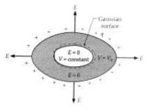
Since  $\vec{E} = 0$  inside the conductor, which gives  $q_{in} = 0$ . As the charge inside the cavity is q. So there must be a charge on cavity wall equal and opposite sign to q. If outer phase is initially unchanged there must be change of +q.
