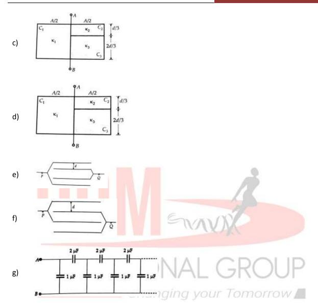
**Question-3:** In the circuit diagram find out the charge a capacitor  $C_1$ ,  $C_2$  and  $C_3$ .
