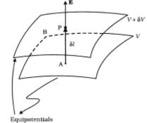
$dV \! \rightarrow \! \text{Decrease}$  in potential in the direction of electric intensity  $\vec{E}$
