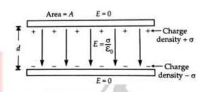
Outer face of 2<sup>nd</sup> plate is earthed because if charged conductor is placed near a earthed conductor its capacity increases.
