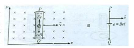
From the diagram, the magnetic force on the free electrons  $\vec{F}_m = -2(\vec{v} \times \vec{B})$  move towards end Q within the rod, hence end Q becomes –ve w.r.t P.
