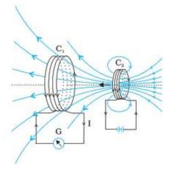
Here the bar magnet is replaced by a second coil C2
