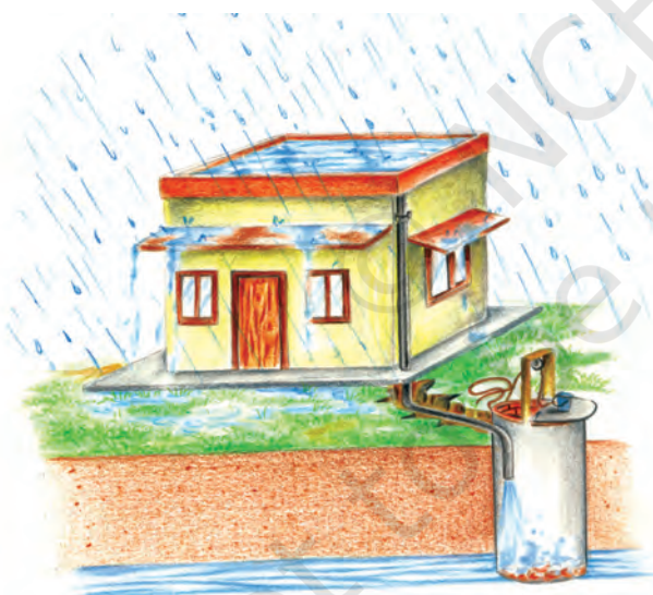
(b) Recharge through Abandoned Dugwell
