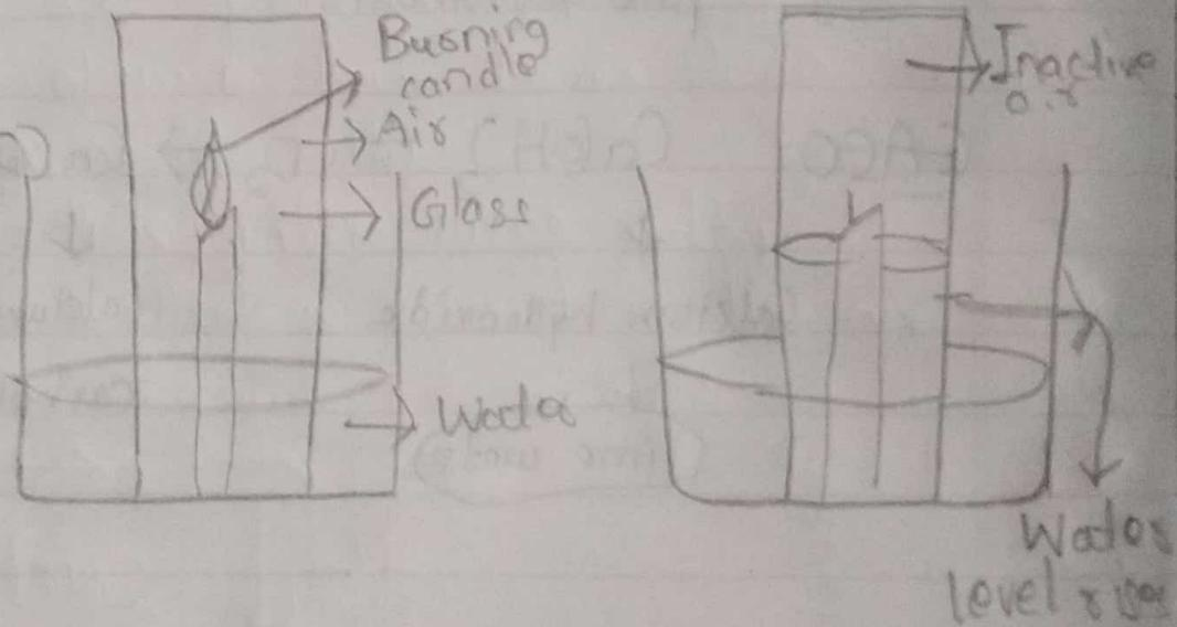
You will observe that the candle continues to burn for sometime and then gets extinguished. The water level rises slightly, i.e. upto  $\frac{1}{5}$ th part of the jar containing air. This part is active, i.e. Oxygen which
