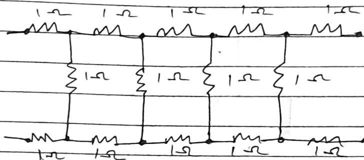
The resistance of each resistor,  $R = 1\Omega$
