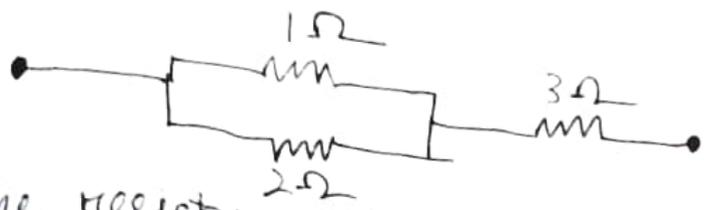
The resistors of resistance  $1\Omega$  and  $2\Omega$  are parallel. Effective resistance  $\frac{1}{R'} = \left[ \frac{1}{1} + \frac{1}{2} \right] = \frac{3}{2}$
