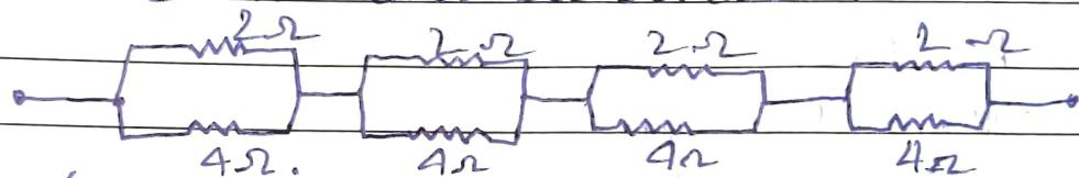
$$R_{eq} (\text{for each loop}) = \frac{2 \times 4}{2+4} = \frac{8}{6} = \frac{4}{3}\ \Omega$$
