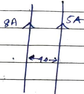
This is an attractive force normal to A and towards B because the direction of the currents in the wires is the same.
