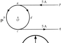
**Question2**: A long wire is bent as shown in the figure. What will be the magnitude and direction of the field at the center O of the circular portion, if a current I is passed through the wire? Assume that the various portions of the wire do not touch at point P
