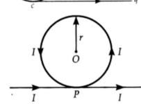
**Question3**: Figure shows a current loop having two circular segments and joined by two radial lines. Find the magnetic field at the center O.
