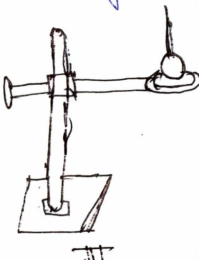
The metal ball is unable to pass through the ring after being heated.
