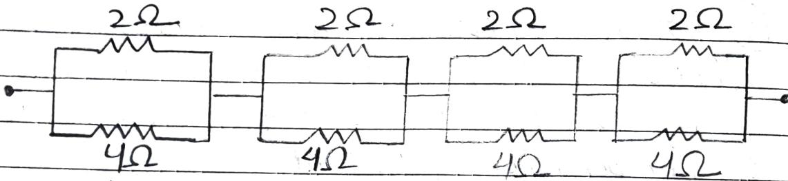
It can be observed that  $2\Omega$  and  $4\Omega$  resistors are connected in parallel in all four loops.
