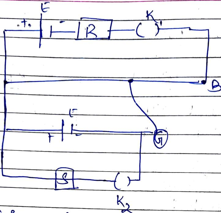
(i) By increasing resistance  $R$  the current through  $AB$  decrease, so potential gradient decrease. Hence a greater length of wire would be needed for balancing the same potential difference so the Null point would shift towards  $B$ .
