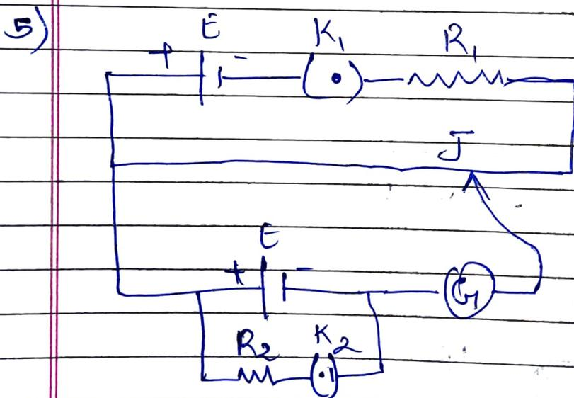
(i)  $R_1$  is increased because the potential gradient would increase.
