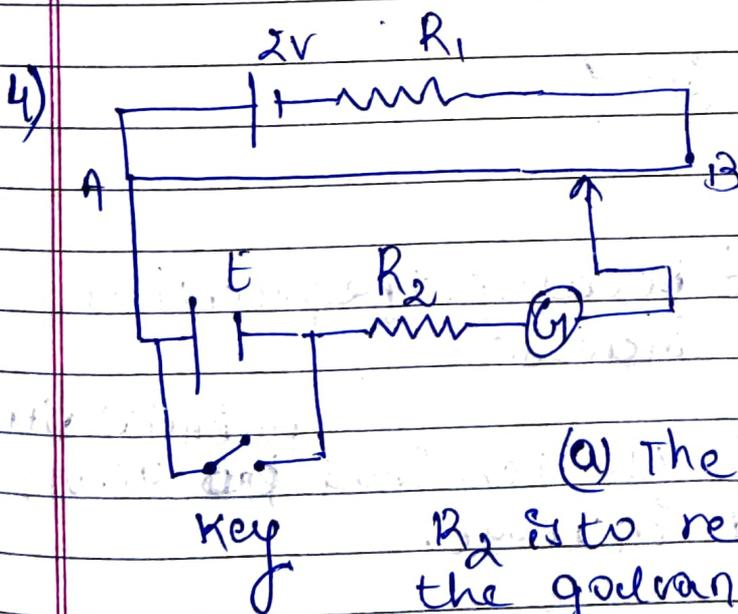
(a) The purpose of high resistance  $R_2$  is to reduce the current through the galvanometer when jockey is far from balance point, this save the galvanometer and the cell from being damaged.
