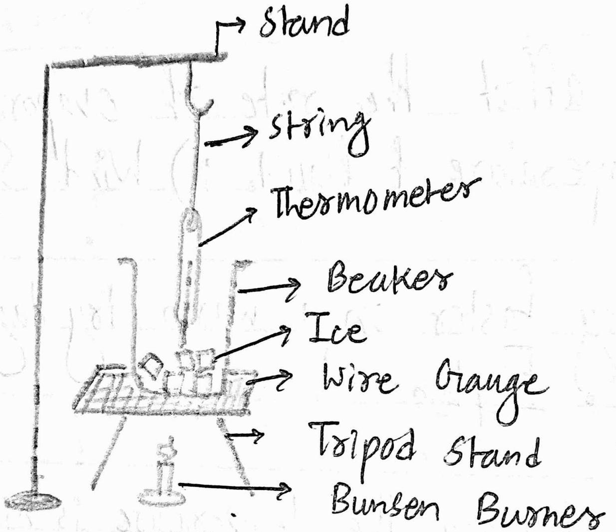
Ans:- Take a beaker and put some ice cubes in it. Keep the beaker and keep it on a wire gauze over a tripod stand. Tie a laboratory thermometer to a stand and tie it with string. Heat the beaker using a bunsen burner. Record the observation of temperature every minute.
