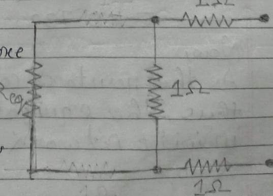
repetition. of the combination of  $1\Omega$  resistors.
