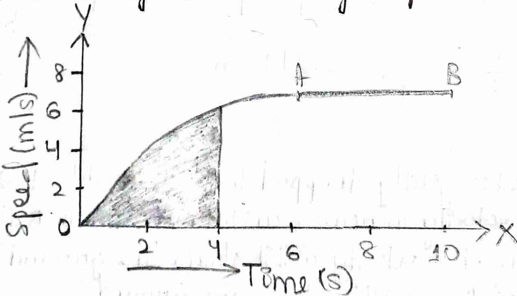
The shaded area which is equal to  $\frac{1}{2} \times 4 \times 6 = 12\text{m}$  represents the distance travelled by the car in the first 4s.
