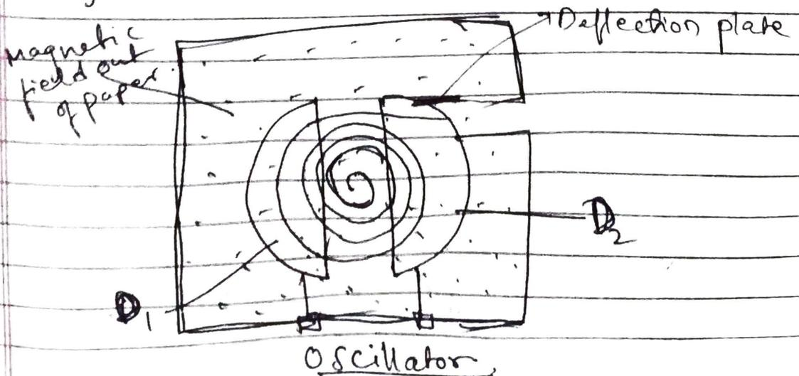
**Principle:** - The charged particle can be accelerated to very high energies by making it pass through moderate electric field by a number of times. This can be done with the help of a  $\perp$  magnetic field which throws the charged particle into a circular motion, the frequency of which doesn't depend on the speed of the particle & the radius of the circular orbit.
