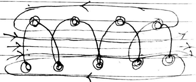
The magnetic field lines of toroid are circular having common centre. Inside a given solenoid, the magnetic field may be made strong by: (i) passing large current and (ii) using laminated coil of soft iron.
